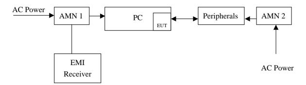
The EUT are connected to the main power through a line impedance stabilization network (LISN). This provides a 50 ohm/50uH coupling impedance for the measuring equipment. The peripheral devices are also connected to the main power through a LISN that provides a 50ohm/50uH coupling impedance with 50ohm termination.
