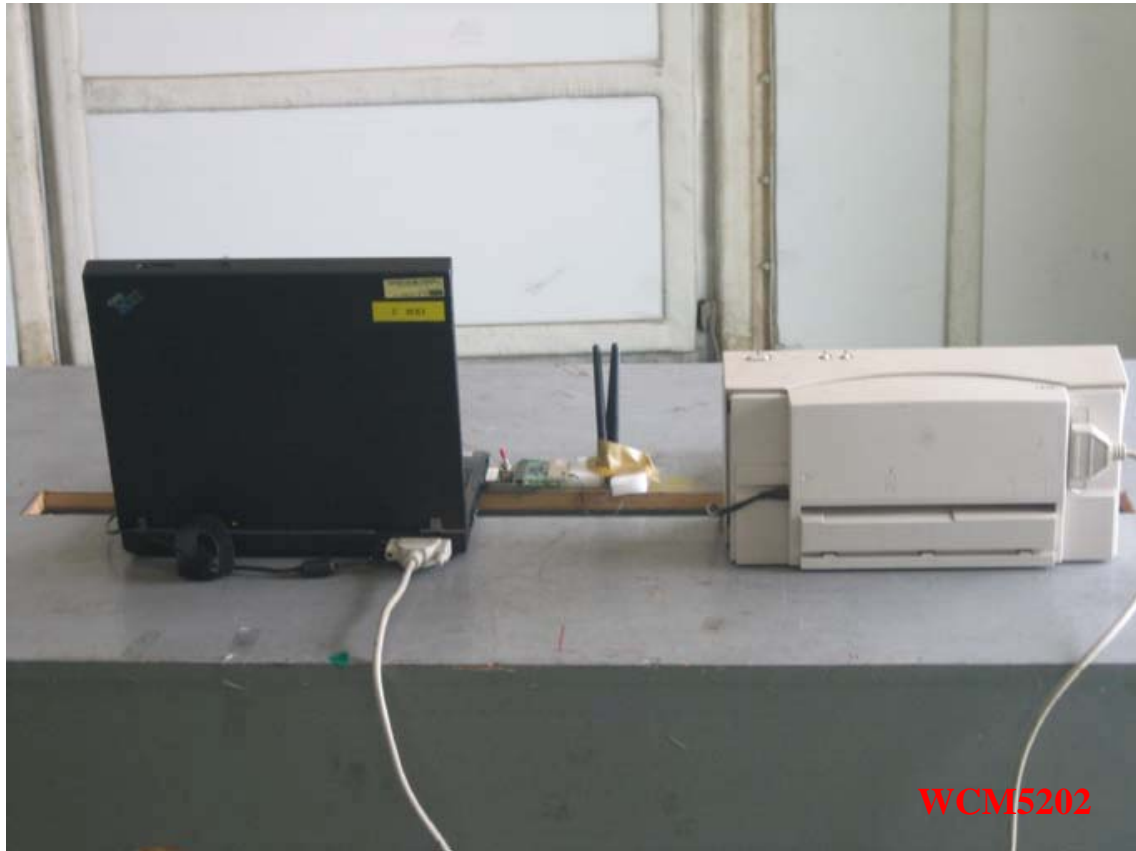
Photo 2: Radiated Emission Test Set-up
