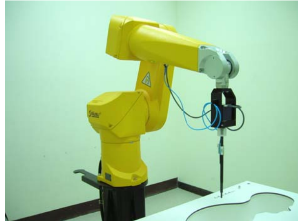
Fig. 5.2 Probe setup on robot
