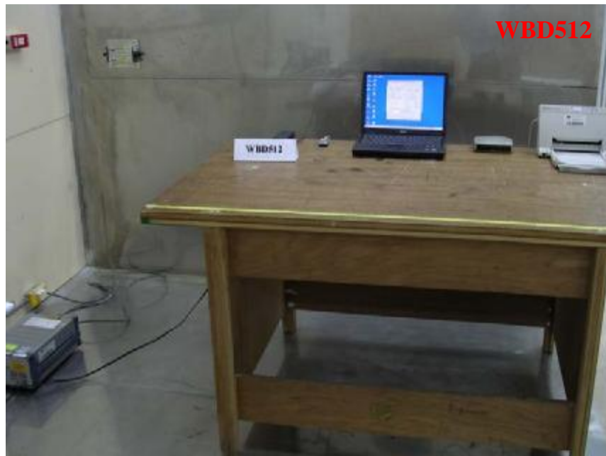
Photo 1: Conducted Test Set-up (front)
