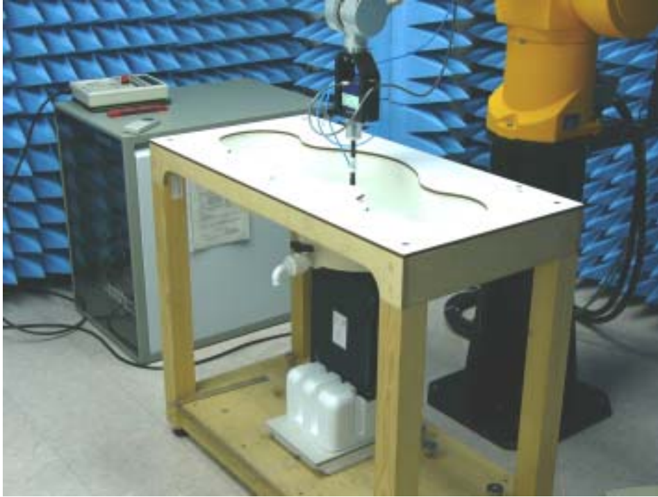
Fig.1 Photograph of the SAR measurement System
