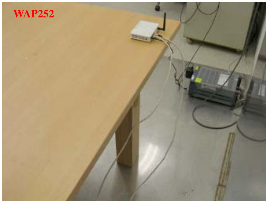
Photo 2: Conducted Emission Test Set-up
