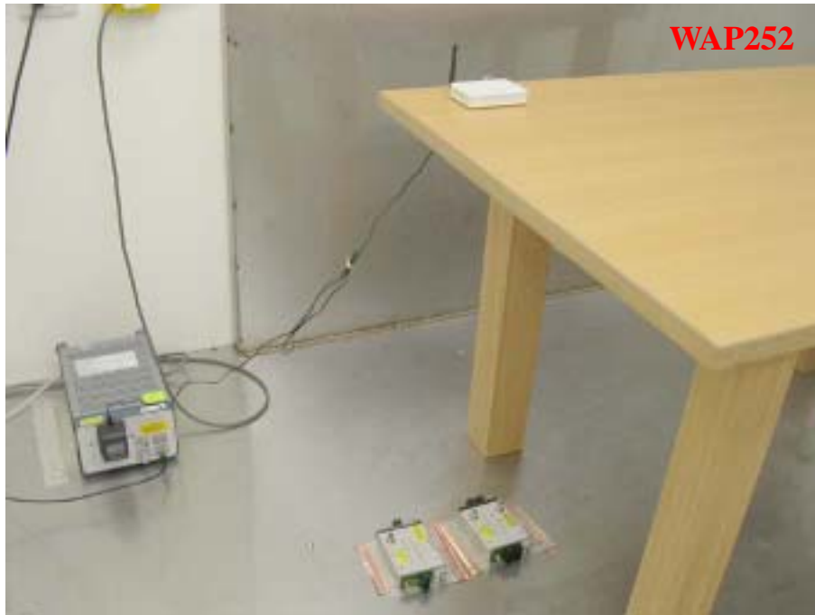
Photo 2: Conducted Emission Test Set-up
