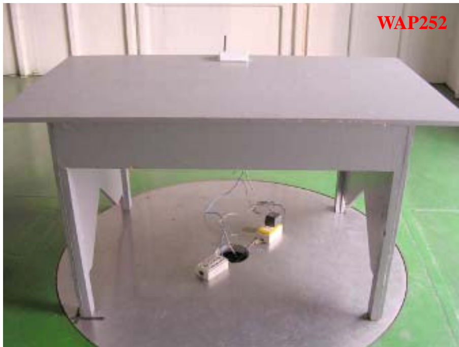
Photo 2: Radiated Emission Test Set-up
