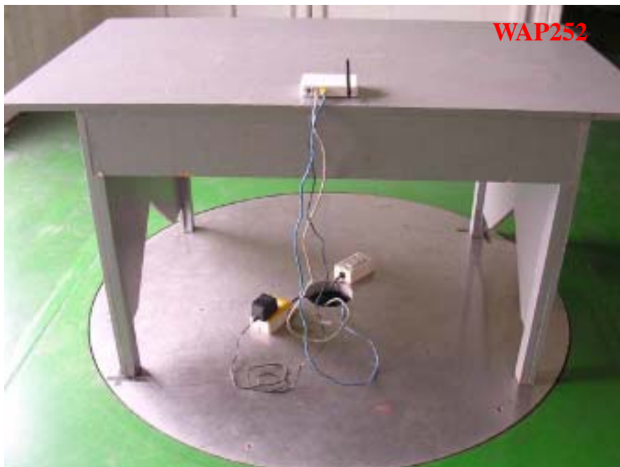
Photo 2: Radiated Emission Test Set-up
