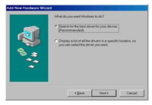
Insert the device driver disk into the floppy disk drive on your system. Select Floppy disk drives and click Next. Windows will search for the drivers for what the new device needs.
