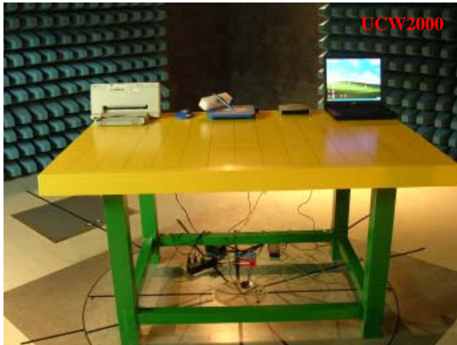
Photo 2: Radiated Emission Test Set-up
