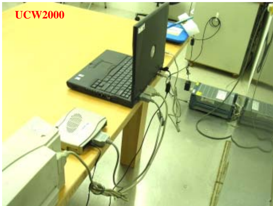
Photo 2: Conducted Emission Test Set-up
