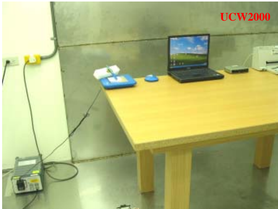
Photo 2: Conducted Emission Test Set-up
