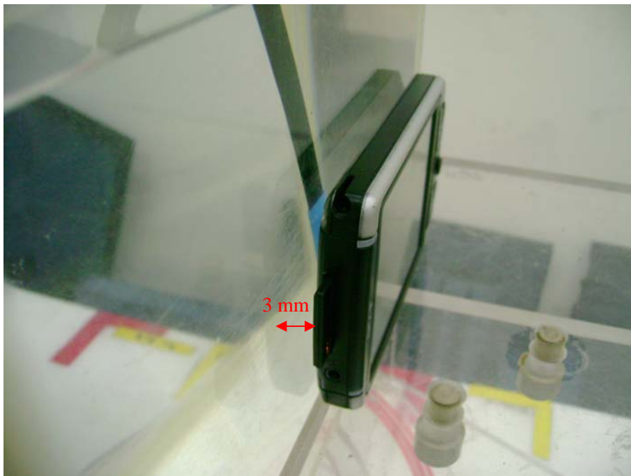
EUT rear to phantom, 0 mm separation of PDA– Zoom In (EUT rear side 3mm to phantom)
