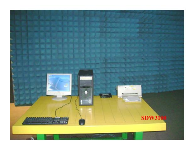
**Photo 2: Radiated Emission Test set-up photo**
