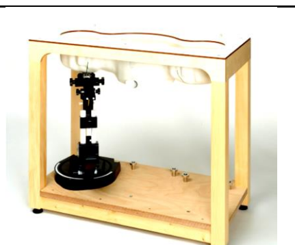
Fig 5.8 Photo of SAM Phantom
