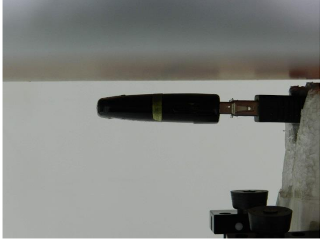
USB Cable Plug-in for USB Configuration 2 (Horizontal Down, Test Separation 5 mm)
