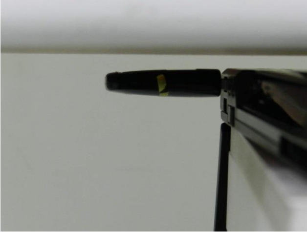
Direct Laptop Plug-in for USB Configuration 1 (Horizontal Up, Test Separation 5 mm)
