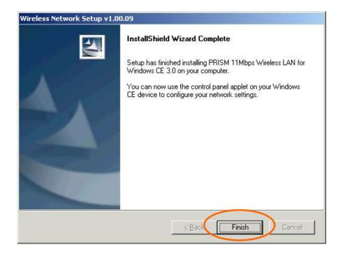
7. You can now insert the Wireless CompactFlash Card into the PDA. Then use the **Settings** on your Windows CE to configure the network settings.
