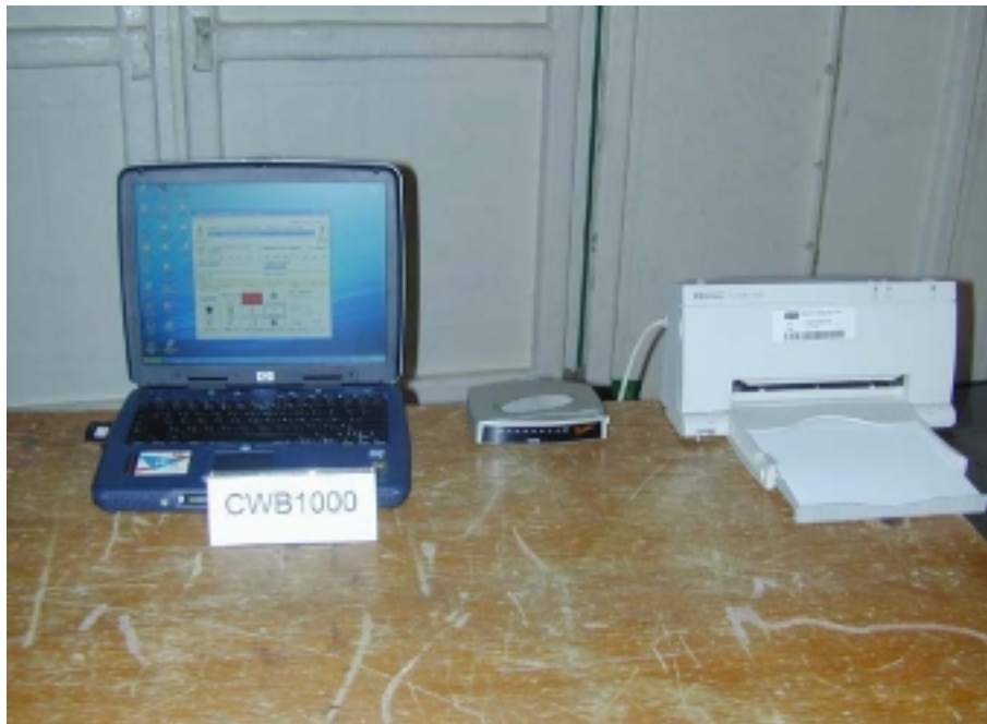
Photo 1: Radiated Emission Test Set-up (front)
