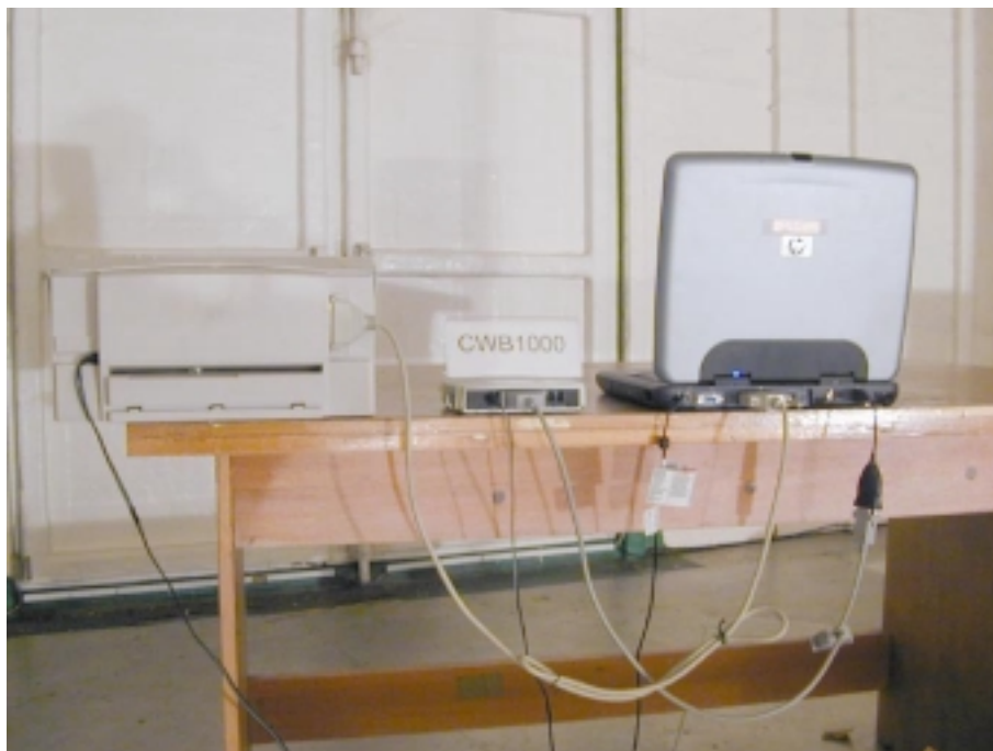
Photo 2: Radiated Emission Test Set-up (rear)
