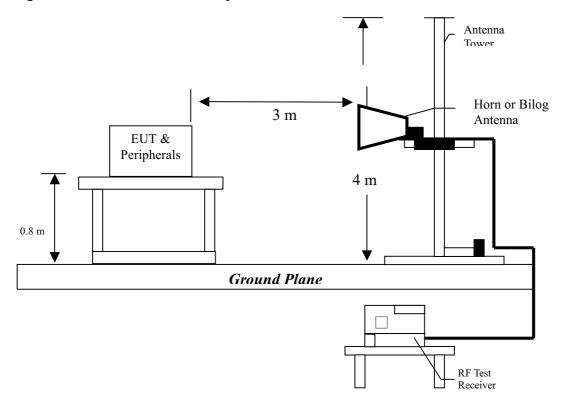
The signal is maximized through rotation and placement in the three orthogonal axes. Radiated emission measurements were performed from 30MHz to 25GHz. Spectrum Analyzer Resolution Bandwidth is 100kHz or greater for frequencies 30MHz to 1GHz, 1MHz – for frequencies above 1GHz.
