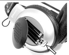
1. Press the battery compartment Cover-Release button on the headset to open the cover and insert two 1.5volt, AAA batteries.
