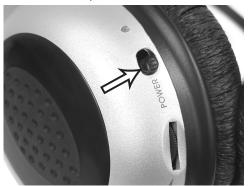
3. Slide the Headset power switch on, the LED light will turn green.
