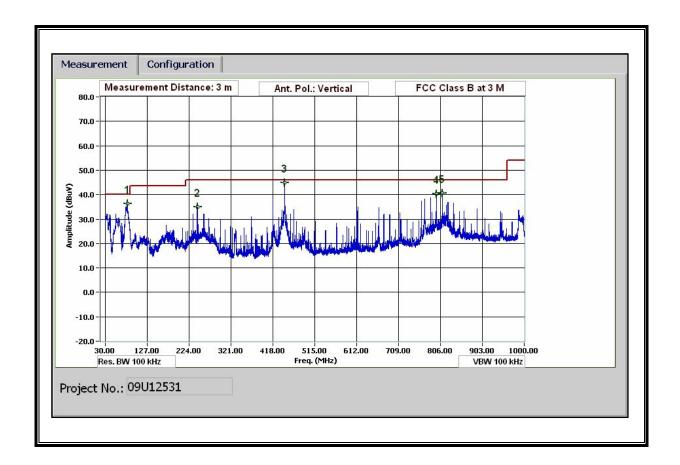
Note: Measurements in this frequency range are made simultaneously on both Source and Sink modules.
