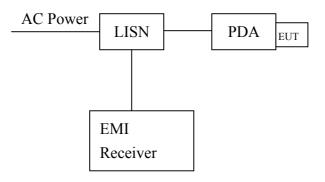
The EUT are connected to the main power through a line impedance stabilization network (LISN). This provides a 50 ohm/50uH coupling impedance for the measuring equipment. The peripheral devices are also connected to the main power through a LISN that provides a 50ohm/50uH coupling impedance with 50ohm termination.
