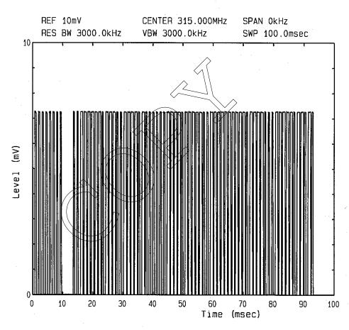
The above waveform indicates the case when field stength averaged over 100 milliseconds was maximum value. In order to obtain the peak to average factor, calculation of the period of total on-time was computed by personal computer. Results was obtaind by following.
