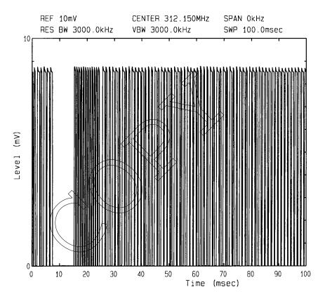
The above waveform indicates the case when field stength averaged over 100 milliseconds was maximum value. In order to obtain the peak to average factor, calculation of the period of total on-time was computed by personal computer. Results was obtaind by following.
