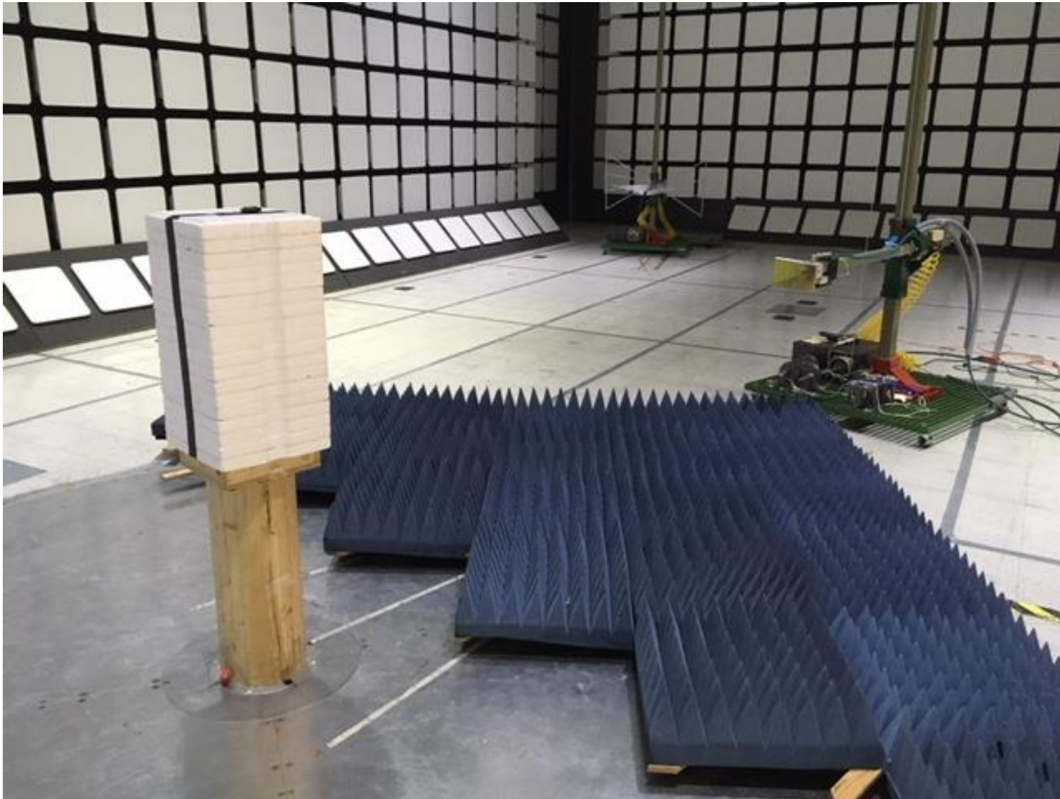
Figure 1 – Radiated Test Setup, >1 GHz
