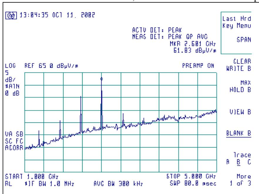
Signature Scans of the Occupied Bandwidth, with antenna in Horizontal polarization
