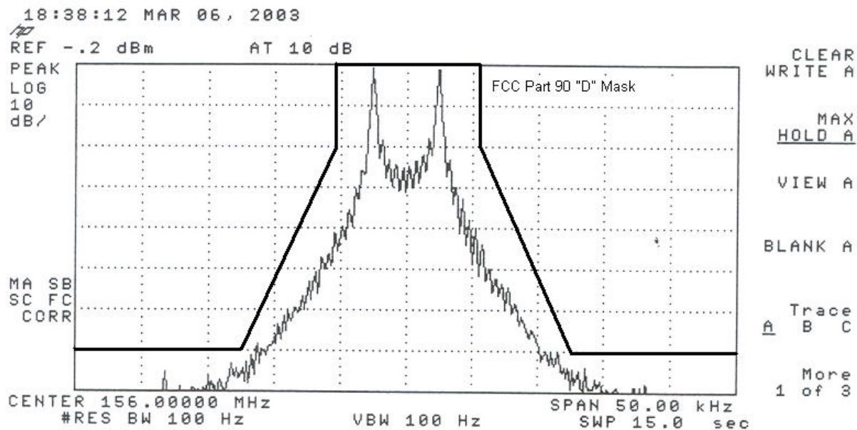
Occupied Bandwidth, 1200 BAUD, POCSAG MODE, Narrowband
