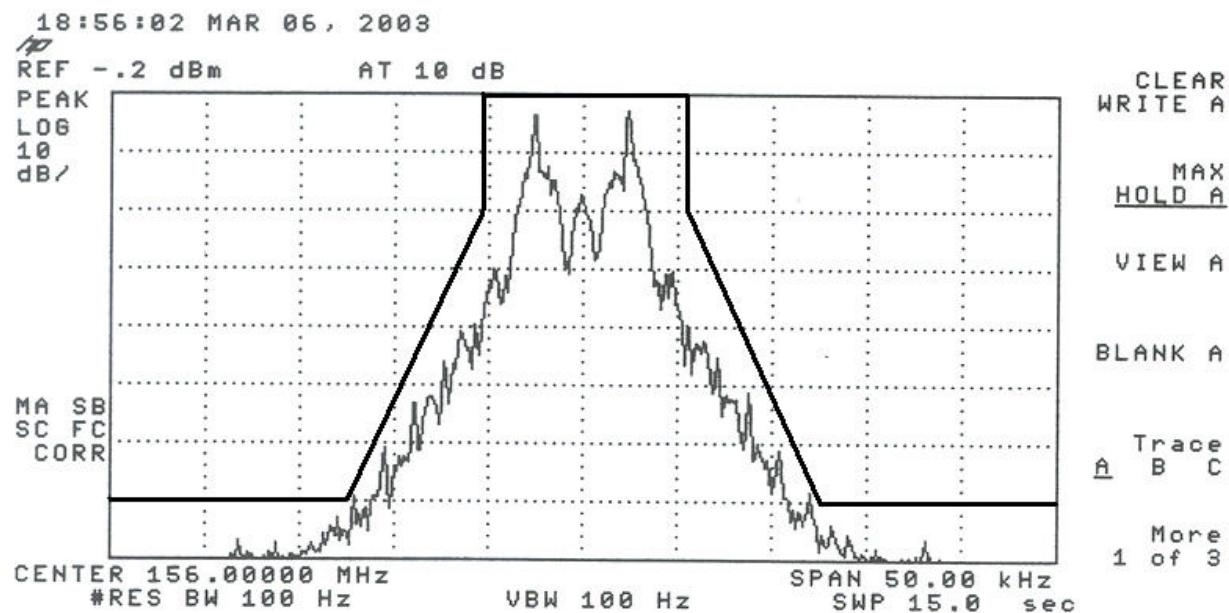
Occupied Channel Bandwidth, 600 BAUD, GOLAY (POCSAG MODE), Narrowband
