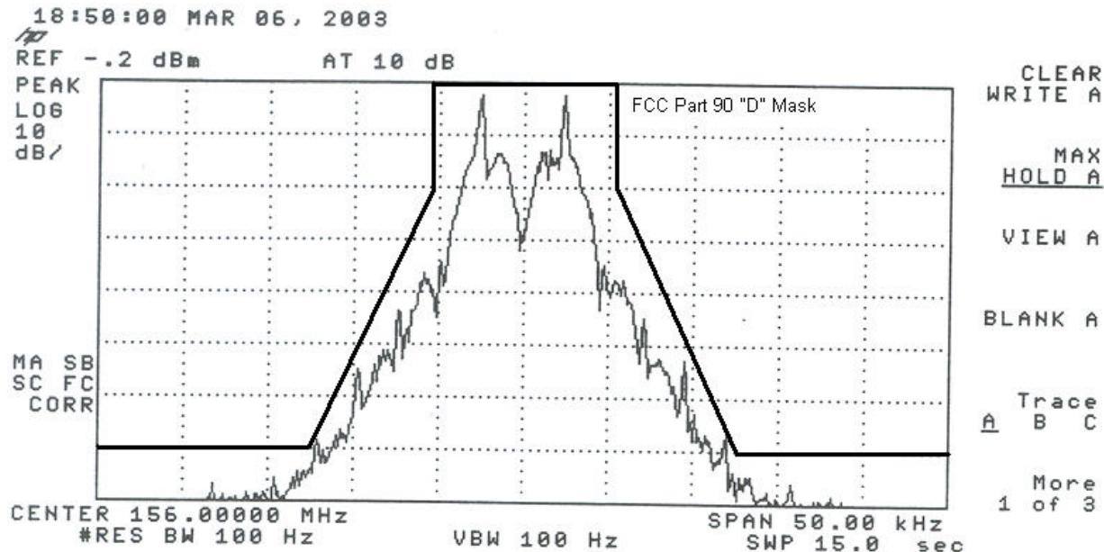
Occupied Bandwidth, 1600 baud 2 Level FLEX MODE, Narrowband
