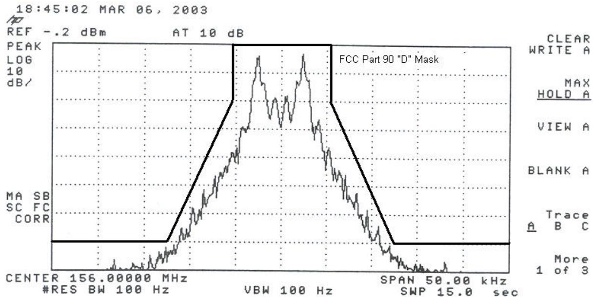
Occupied Channel Bandwidth 2400 BAUD, POCSAG MODE, Narrowband
