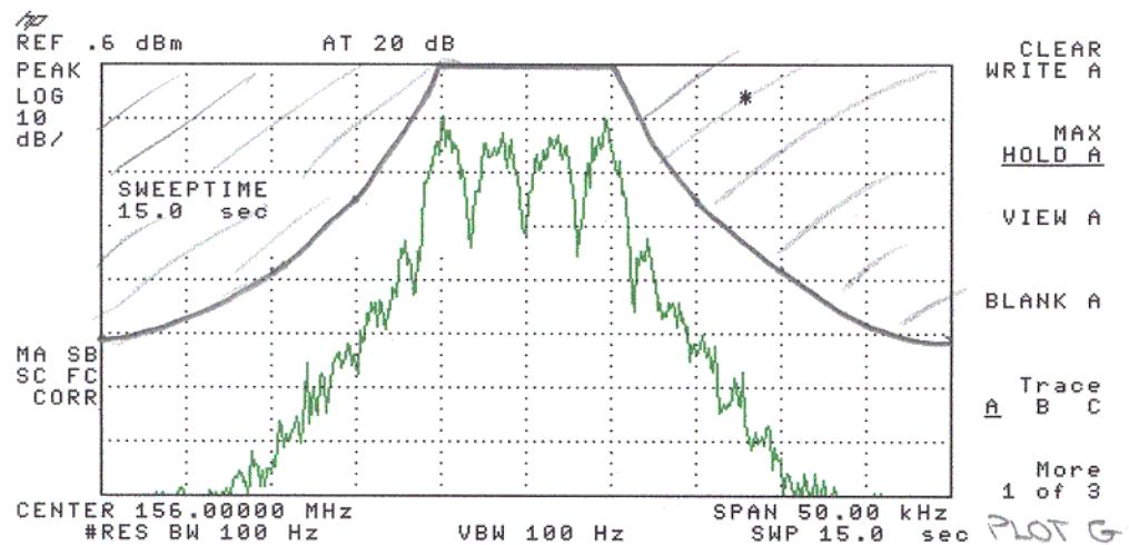
4.3.8 Occupied channel Bandwidth, 1600 BAUD, FLEX, 2 LEVEL
