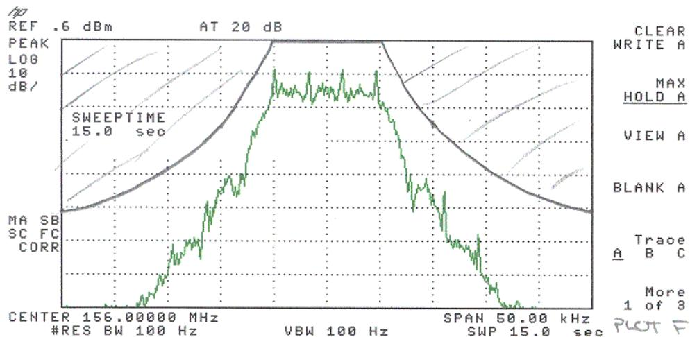
4.3.7 Occupied Channel Bandwidth, 3200 BAUD, FLEX, 4 LEVEL
