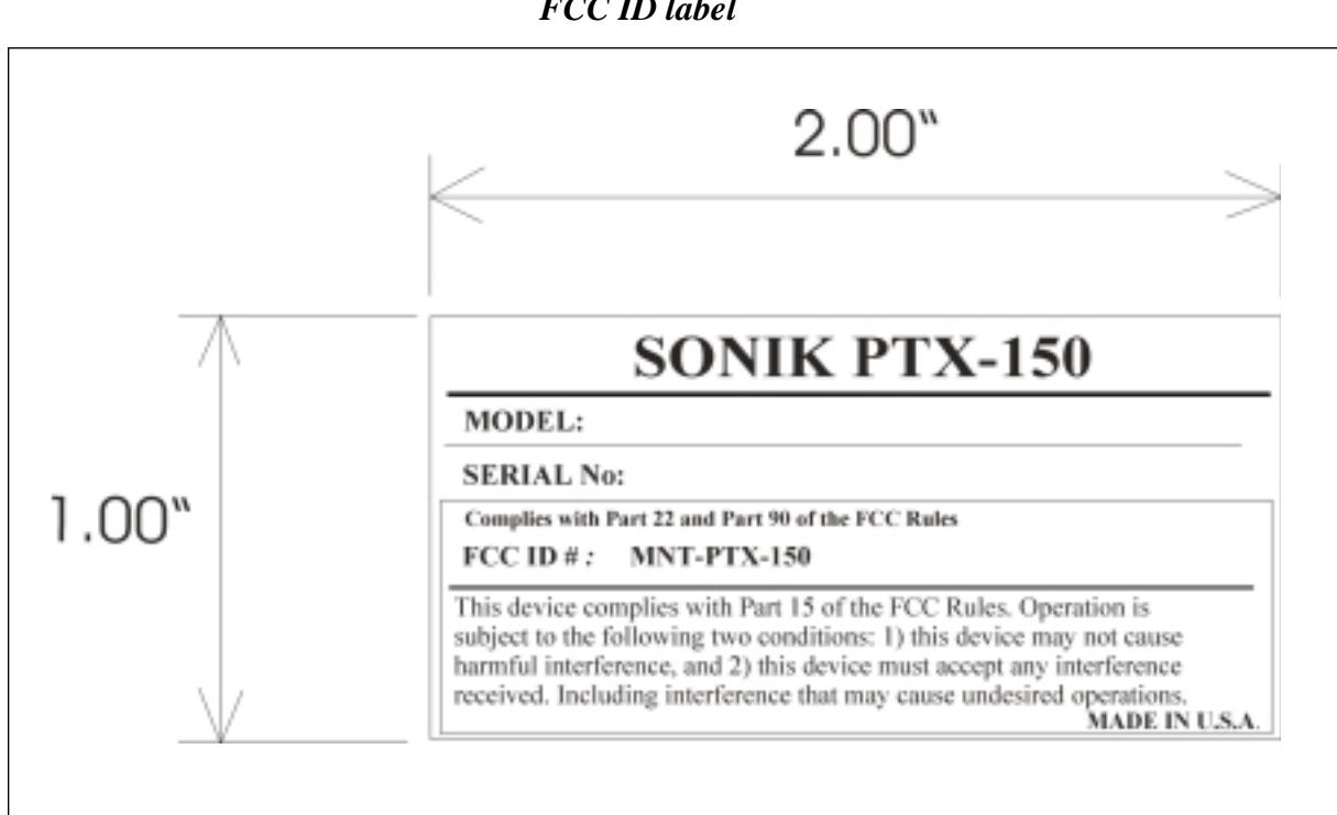
*Location of label is below the "External Frequency" BNC jack and directly to the left of the "LIU" and "RS-232" connectors on the rear panel. The label is to be placed as not to obstruct any of the other labels or markings.*
