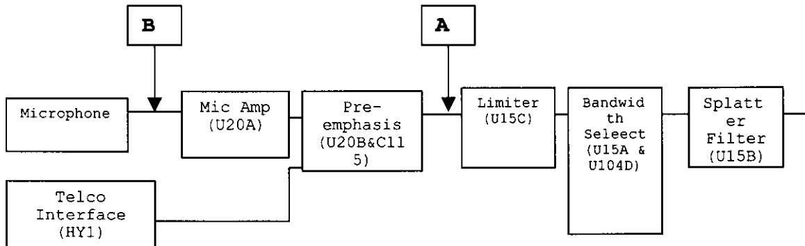
The output of the audio pre-emphasis goes to a circuit that sets the limited voltage to either time 0.5 or time 0.25. The output of the Bandwidth select circuit goes to the splatter filter and then to the transmitter's modulation circuit in the VCO.
