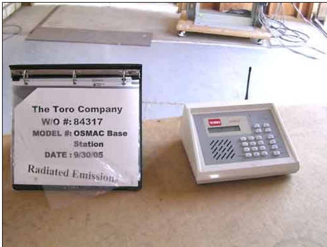
Radiated Emissions - Front View
