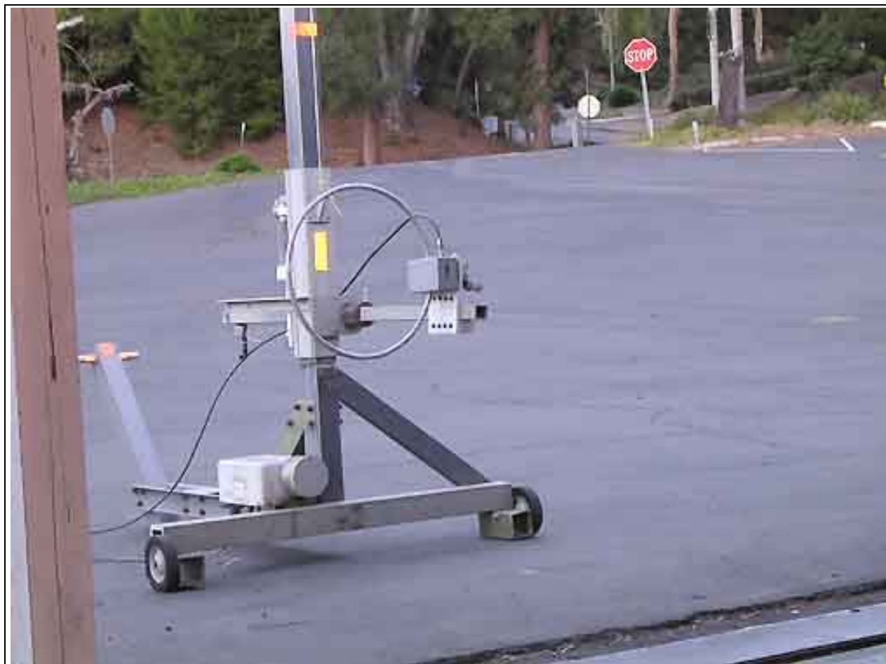
Radiated Emissions - Back View Loop Antenna
