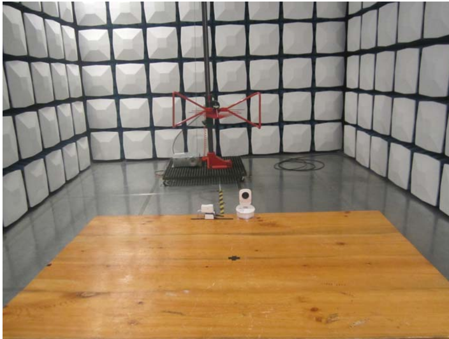
Radiated Emission –Front View (Below 1G)
