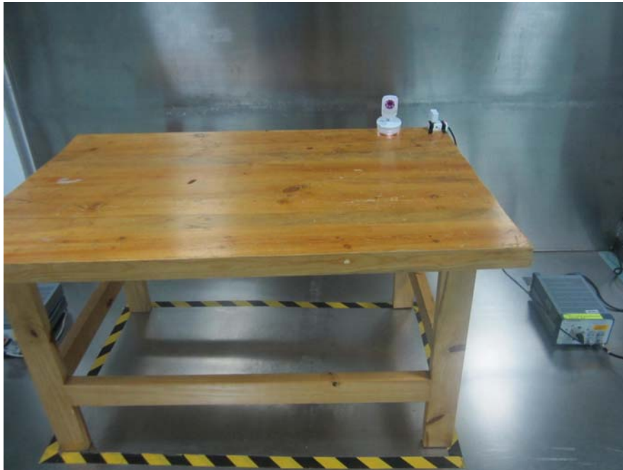
Conducted Emission--Front View
