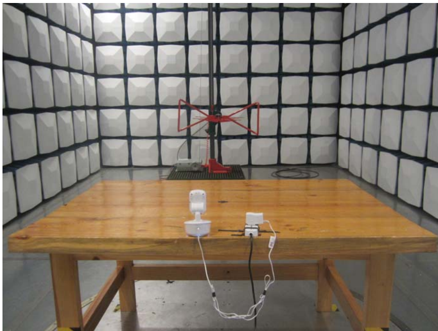
Radiated Emission –Rear View (Below 1G)
