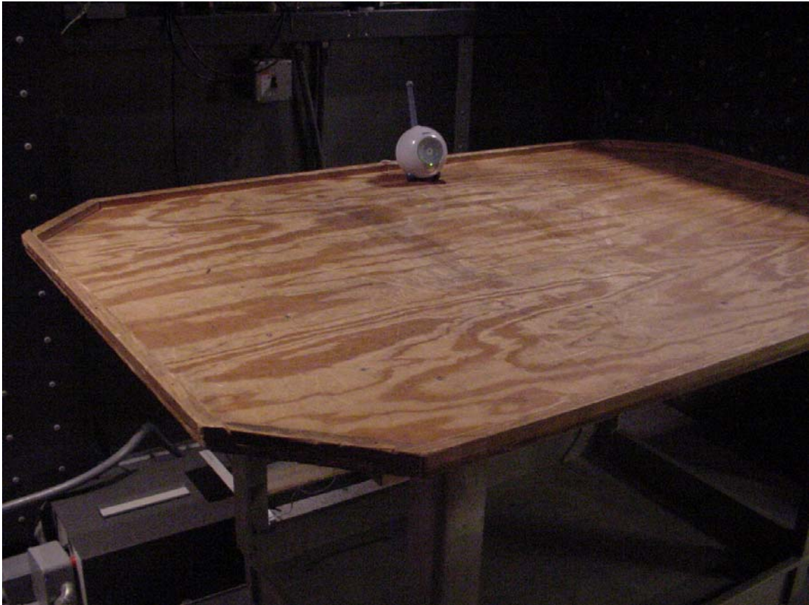
Conducted Test Setup Front
