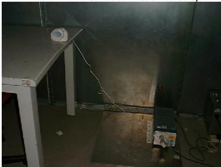
Measurement of Conducted Emission Test Set Up
