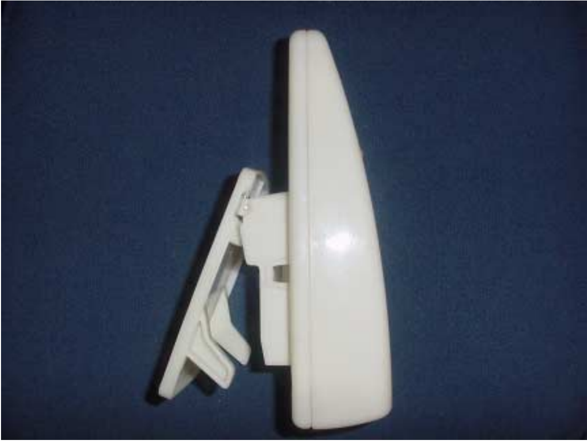
Side View of EUT with EUT configured in Table Top setup, the stand can also be adjusted vertical to allow wall mounting.
