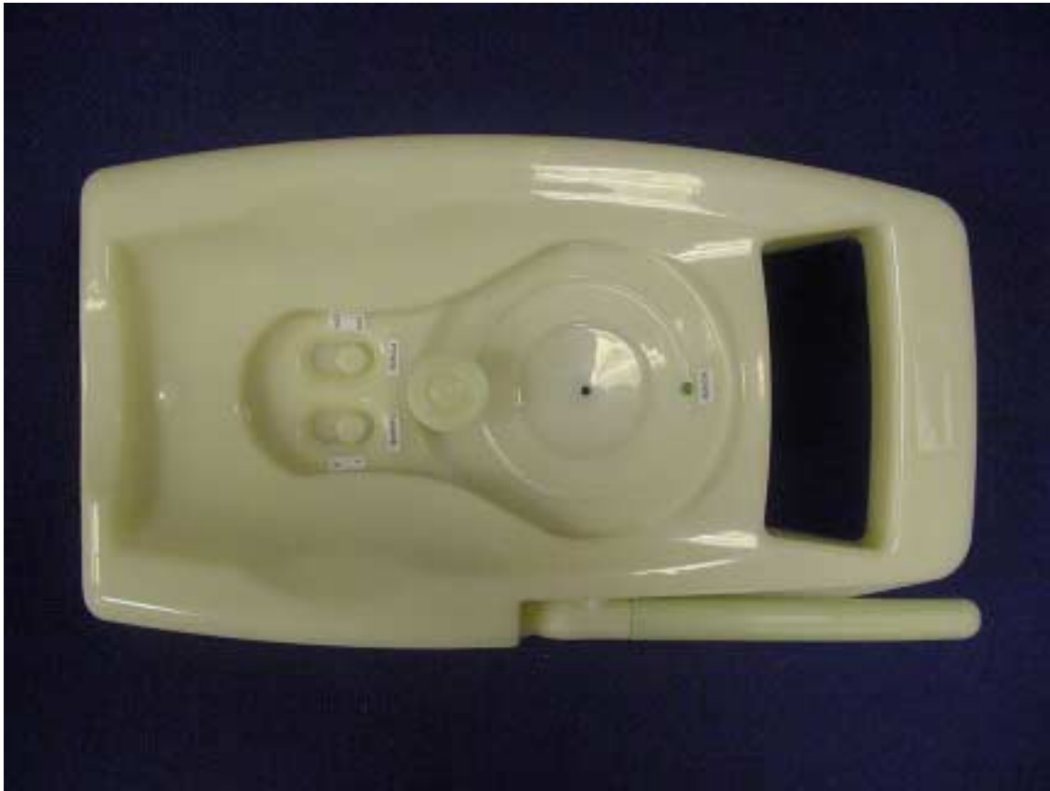
Front View, showing On/Off and Channel Selector switches. Antenna is at bottom right.
