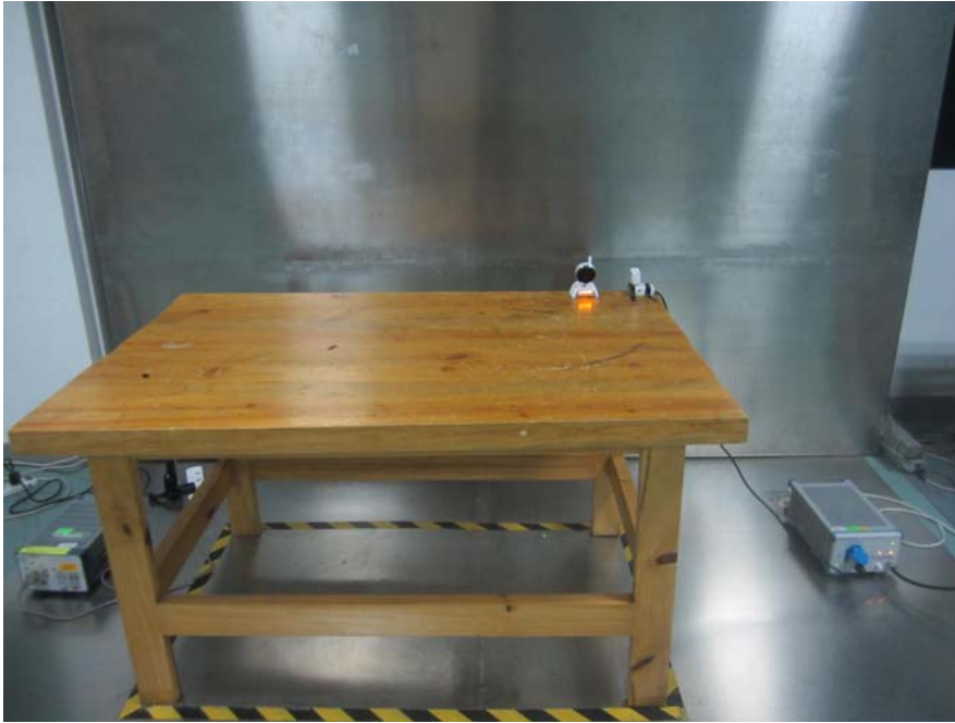
Conducted Emission--Front View
