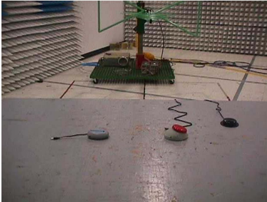
Radiated Emissions Test Configuration
