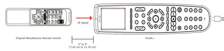
The Pro24.r is capable of capturing infrared codes from original equipment manufacturer remote controls. This IR learning capability is designed to work together with the Pro Control Studio library manager software. To capture infrared codes, follow the steps listed below:
