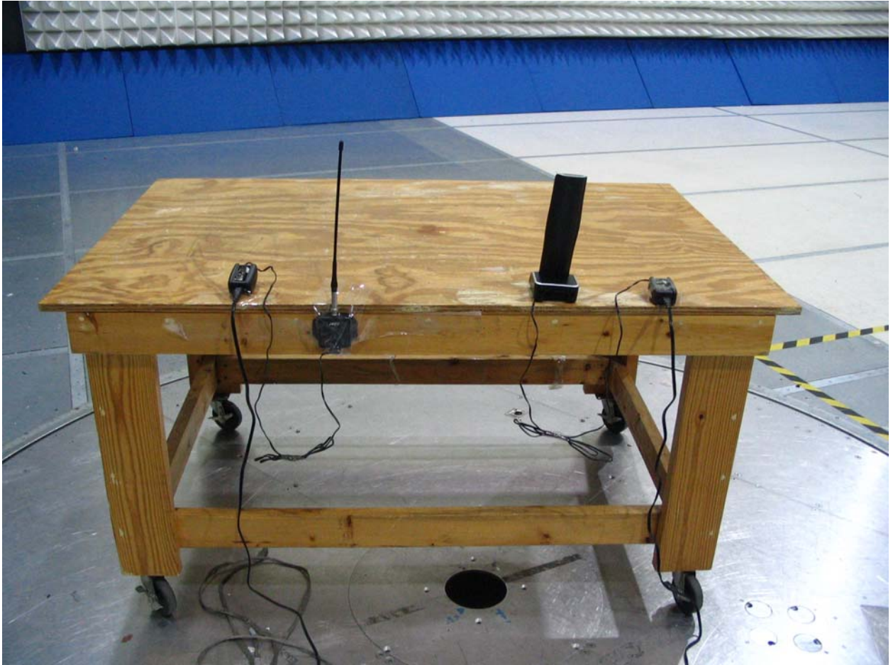
Figure 1: Back Side of Emissions Setup (Remote in Charging Base)
