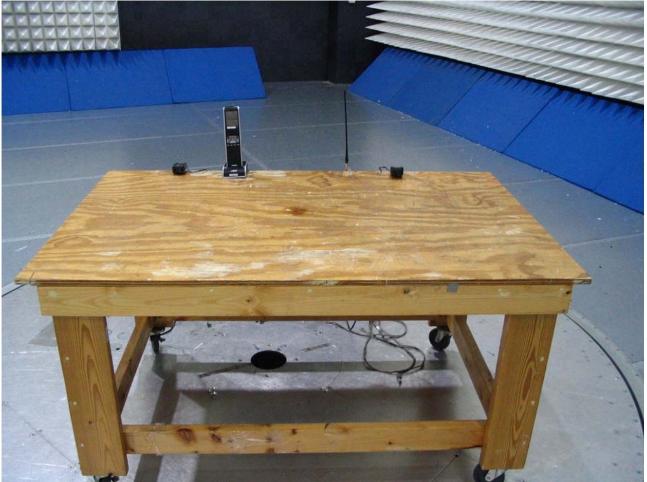
Figure 2: Front Side of Emissions Setup (Remote in Charging Base)
