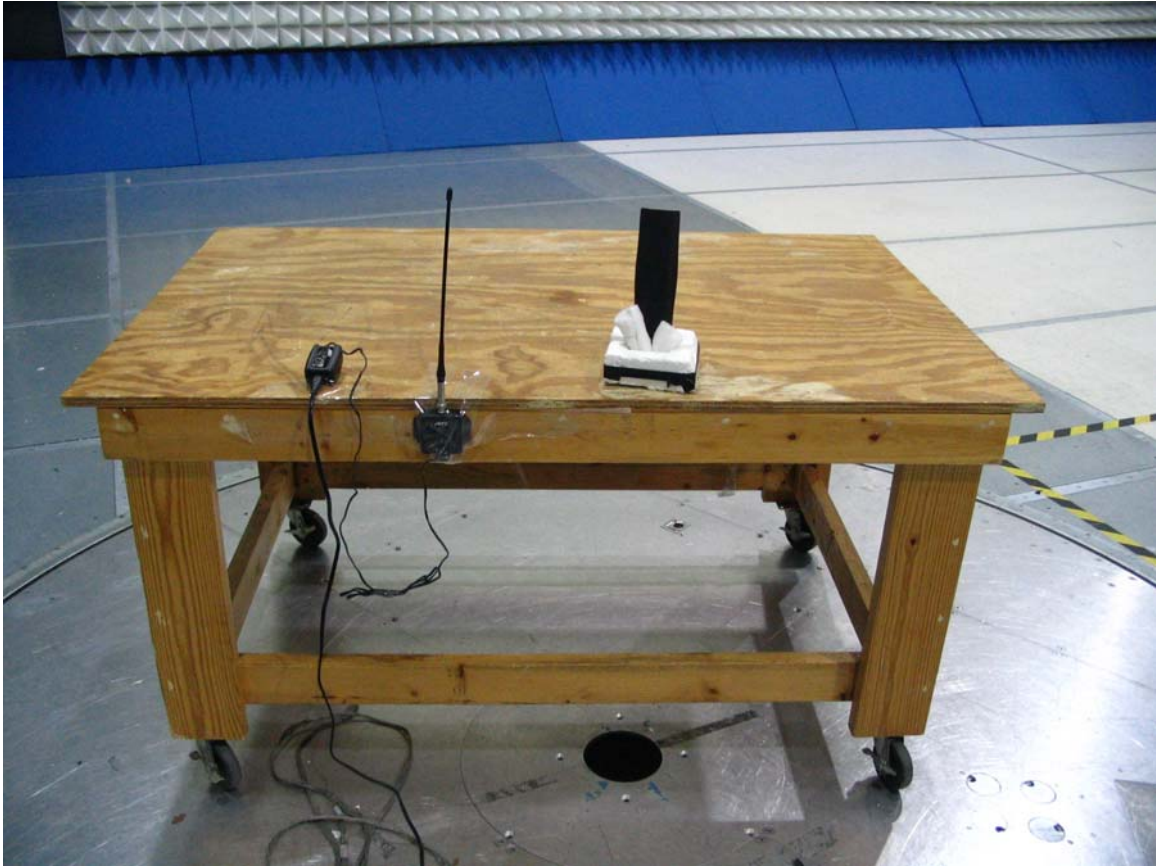
Figure 3: Emissions Test Setup (Transmitting)
