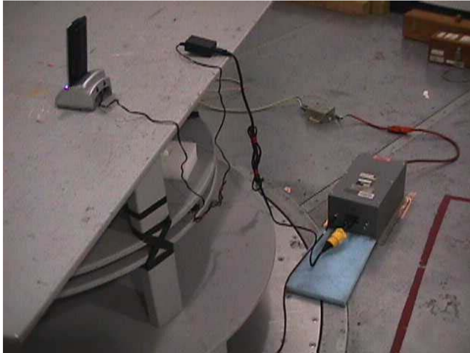
Line Conducted Emissions Test Configuration (T3 Remote Control Charger)
