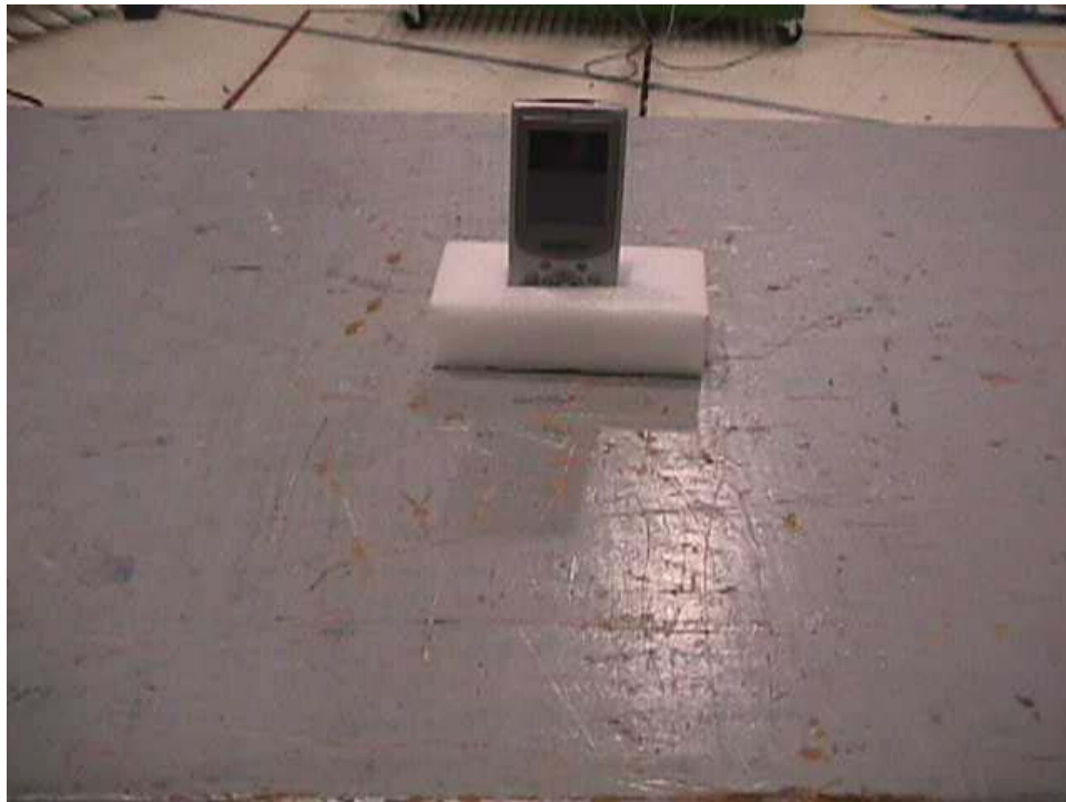
Radiated Emissions Test Configuration (T3 Remote Control Transmitter)
