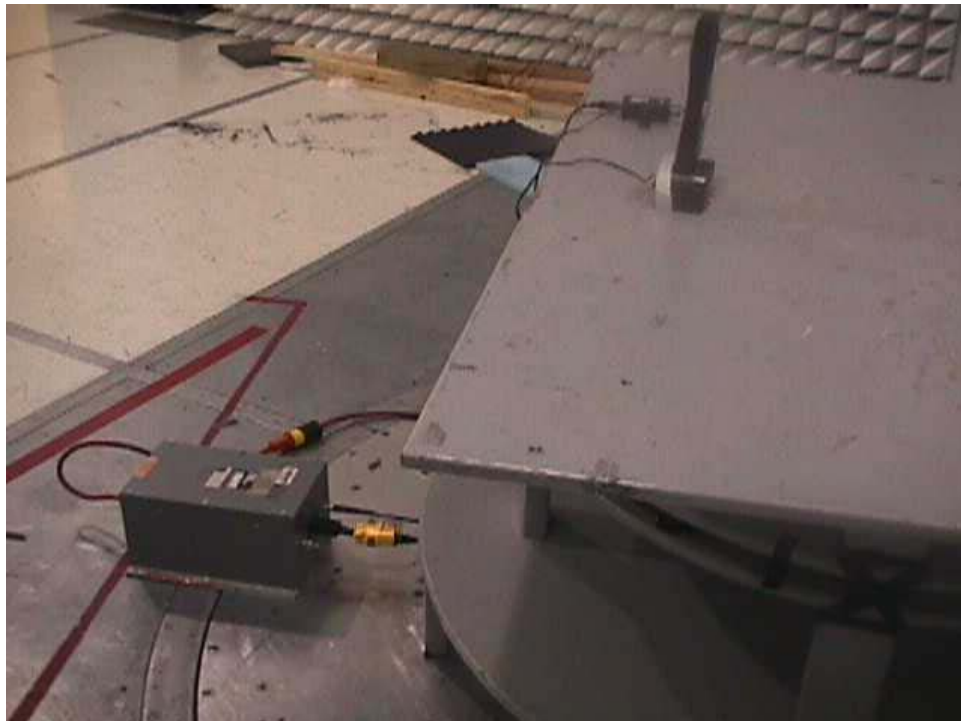
Line Conducted Emissions Test Configuration (ST2 Remote Control Charger)
