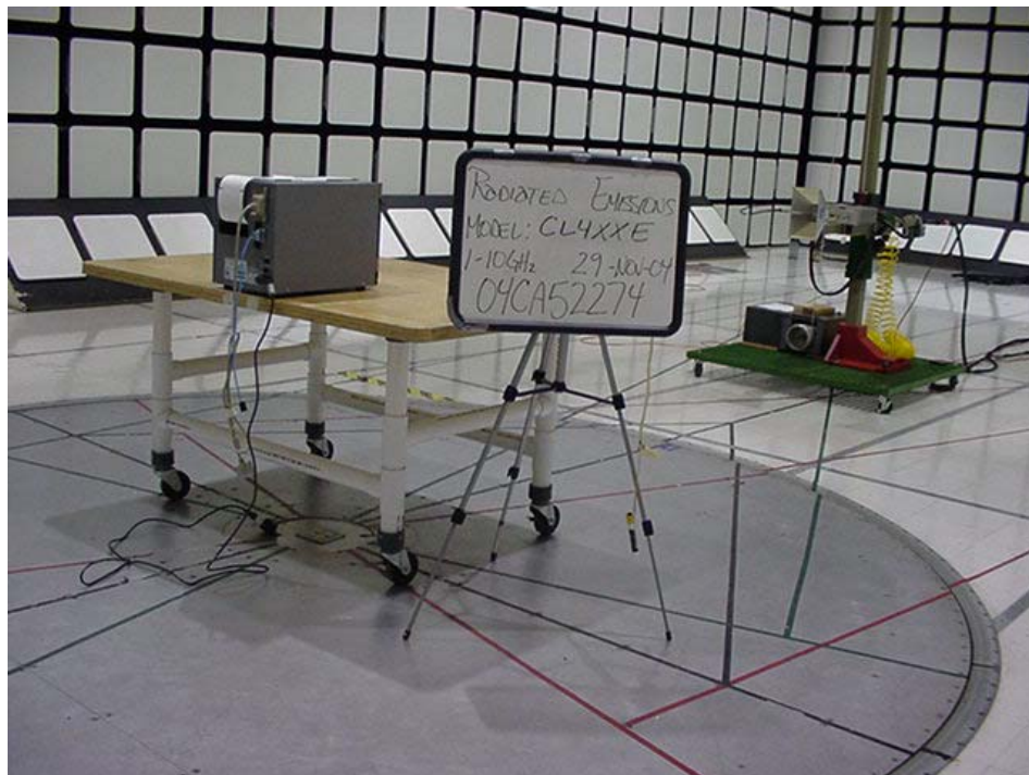
Radiated Emissions Test Setup 1-10 GHz
