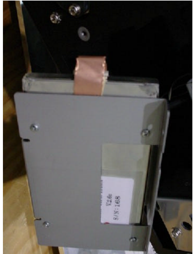
Figure 1.6a Transmitter Ribbon Cable Shielding
