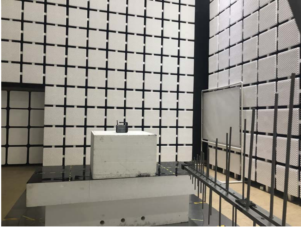
Radiated RF measurement (30 MHz - 1 GHz)
