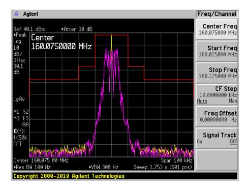
High Power: Audio; 12.5 kHz Channel Spacing
