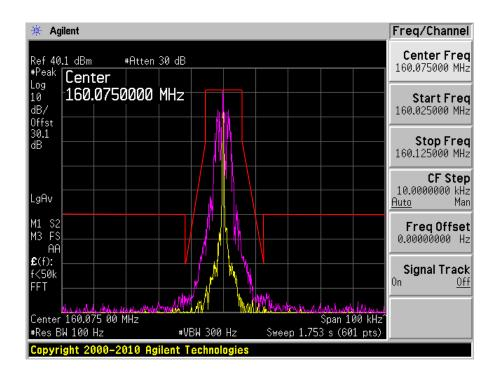
Low Power: Data; 25 kHz Channel Spacing
