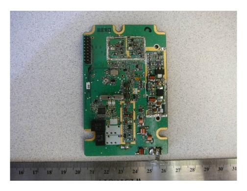
15.12 EUT- RF PCB Board (Unshielded) Bottom View
