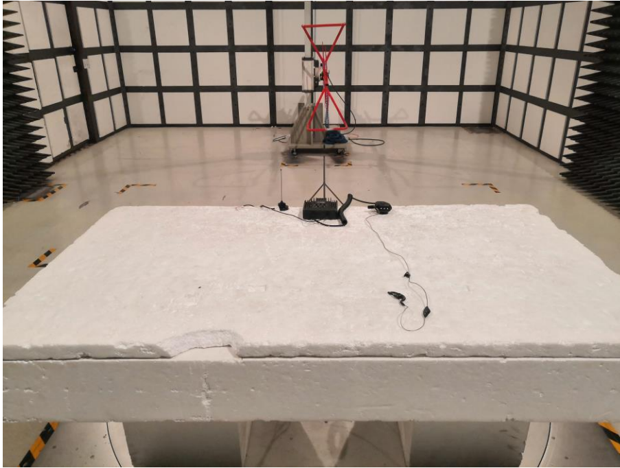
Radiated Disturbances Rear Side (Below 1GHz)
