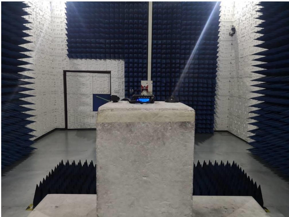
RADIATED EMISSION ABOVE 1G TEST SETUP
