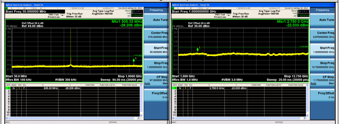
12.5kHz, FM modulation, Assigned Frequency:467.6500MHz, 50W
