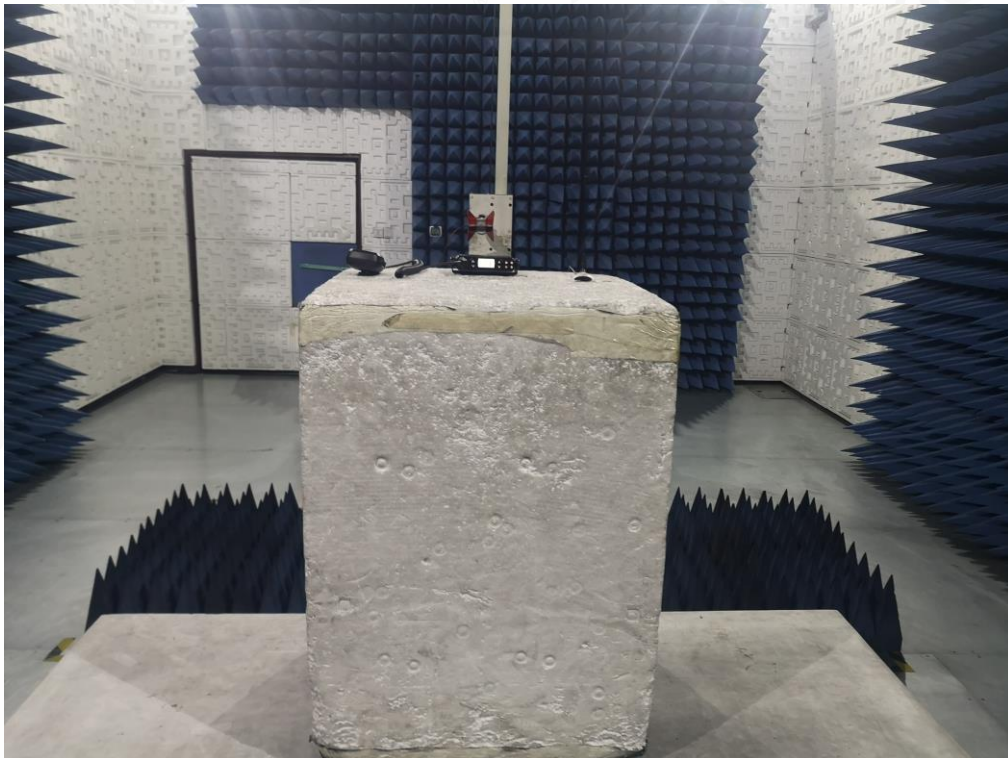
RADIATED EMISSION ABOVE 1G TEST SETUP
