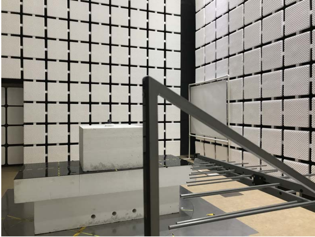
Radiated RF measurement (30 MHz - 1 GHz)
