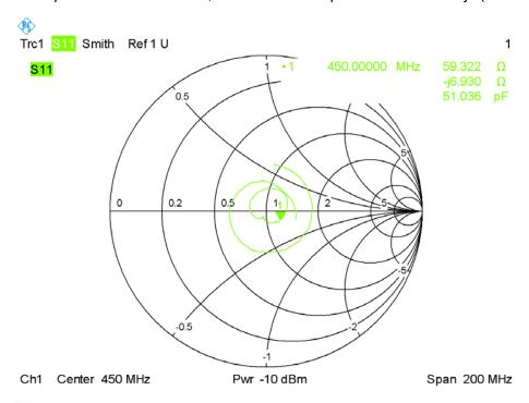
Calibrated return loss: -22.6dB; Measurement return loss: -22.8 dB(within 20%)
