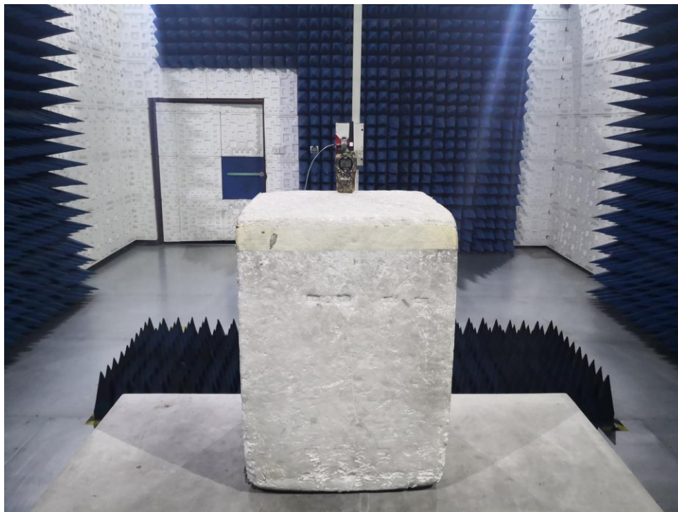
RADIATED EMISSION TEST SETUP ABOVE 1GHz
